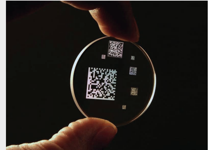
Laser marking. Written directly inside the object (glass) by making refractive index irregularities without damaging the surface
