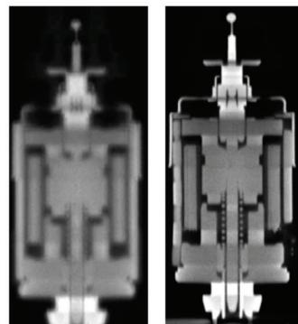
The images above illustrate the superior performance of the HP Technology versus traditional X-Ray. Both images were made using the same power and exposure duration. Due to the smaller focal point of HP Tube, the resolution of the image on the right is clearer and shows far more detail.
